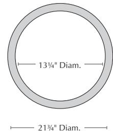
**Materials:** unsaturated polyester resin, sand, stone powder, talc powder, and fiberglass
