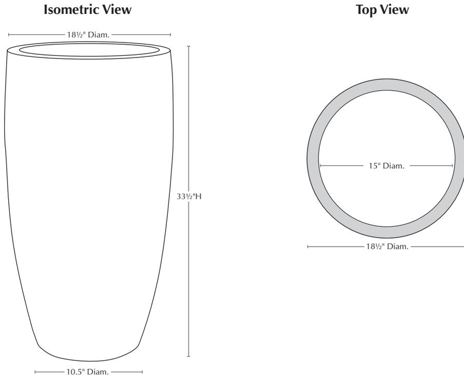
**Materials:** unsaturated polyester resin, sand, stone powder, talc powder, and fiberglass
