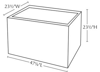
**Materials:** unsaturated polyester resin, sand, stone powder, talc powder, and fiberglass
